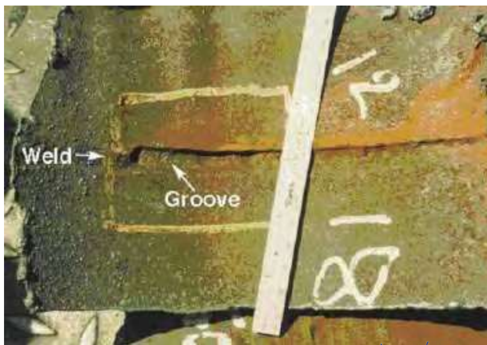
Figure 3-2-1—Localized amine corrosion at the weld found in piping from the reboiler to the regenerator tower in an MEA unit. Many other similar cases were found, some going as deep as half thickness. They were originally found with shear wave UT inspection and mistaken as cracks.
