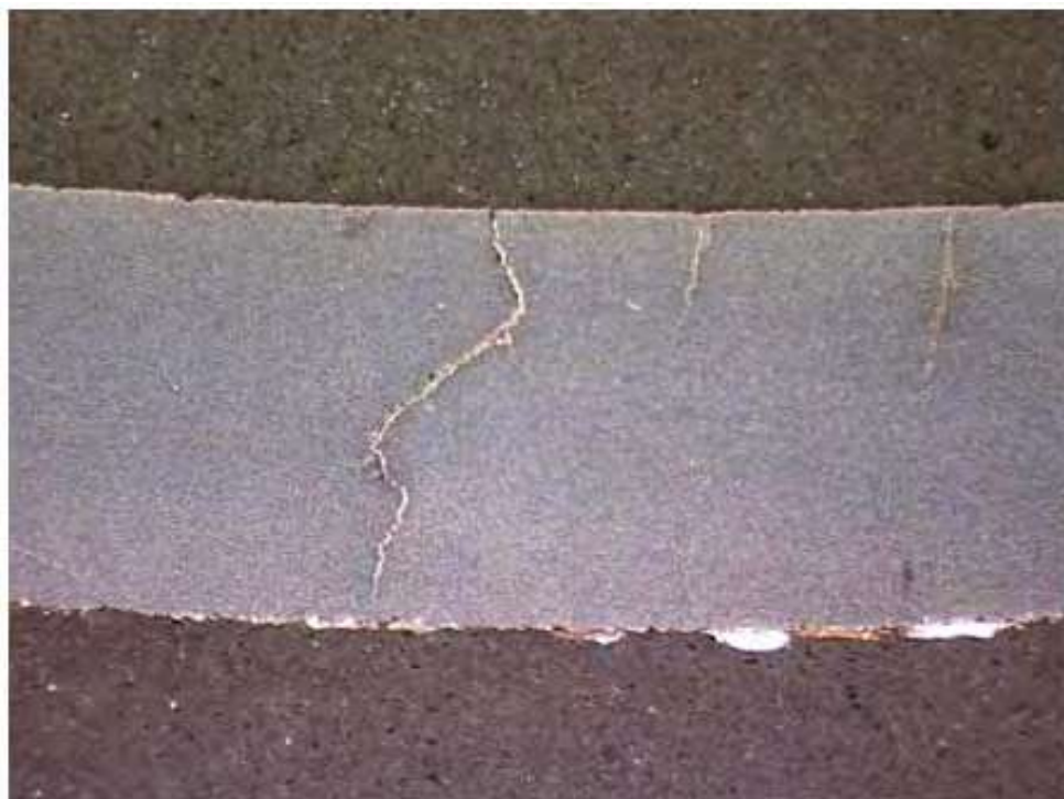
Figure 3-28-7—Transverse cross section of a piping section exposed to fuel ethanol showing multiple crack initiation sites characteristics of SCC.
