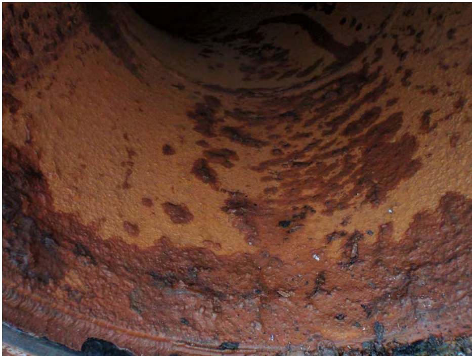
Figure 3-10-2 – Close-up of brine corrosion on flange in Figure 3-10-1.
