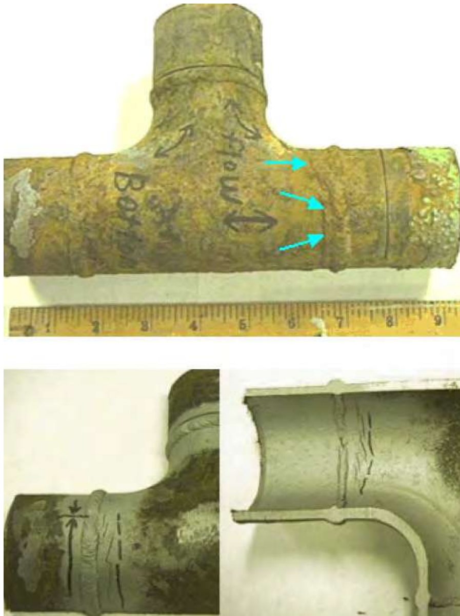
Figure 3-28-5—Ethanol SCC of steel piping in a fuel ethanol system return line/tank transfer line. The top picture shows the crack parallels the pipe-to-tee circumferential weld. The bottom picture shows the inside and outside of the pipe after splitting and cleaning the weld area. Parallel SCC cracks are clearly visible adjacent to the weld.
