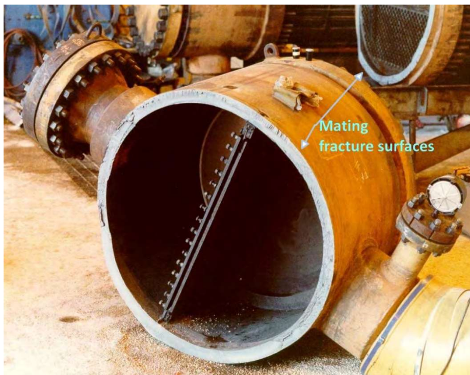
Figure 3-11-3—Brittle fracture of a 2.2-in. wall C-0.5Mo exchanger channel during hydrotest.
