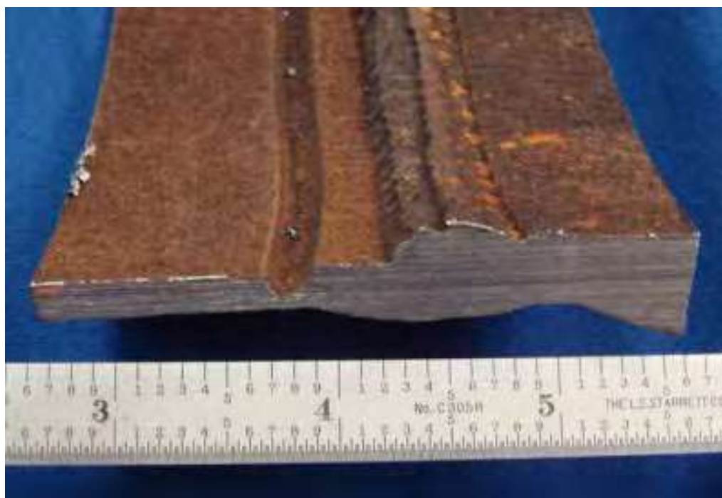
Figure 3-2-2—Hot lean amine corrosion of carbon steel attributed to increased CO 2 content in the MEA solution.
