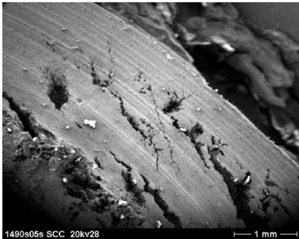
Figure 3-17-6—Cl - SCC on the thread surface of a failed 303 SS bolt.
