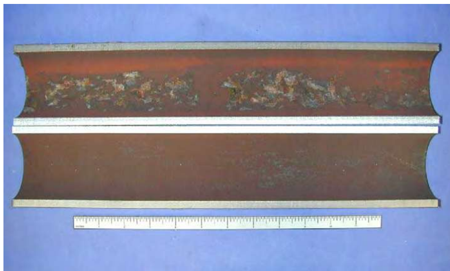
Figure 3-14-1—ID deposits on carbon steel boiler tube with damage due to caustic corrosion.
