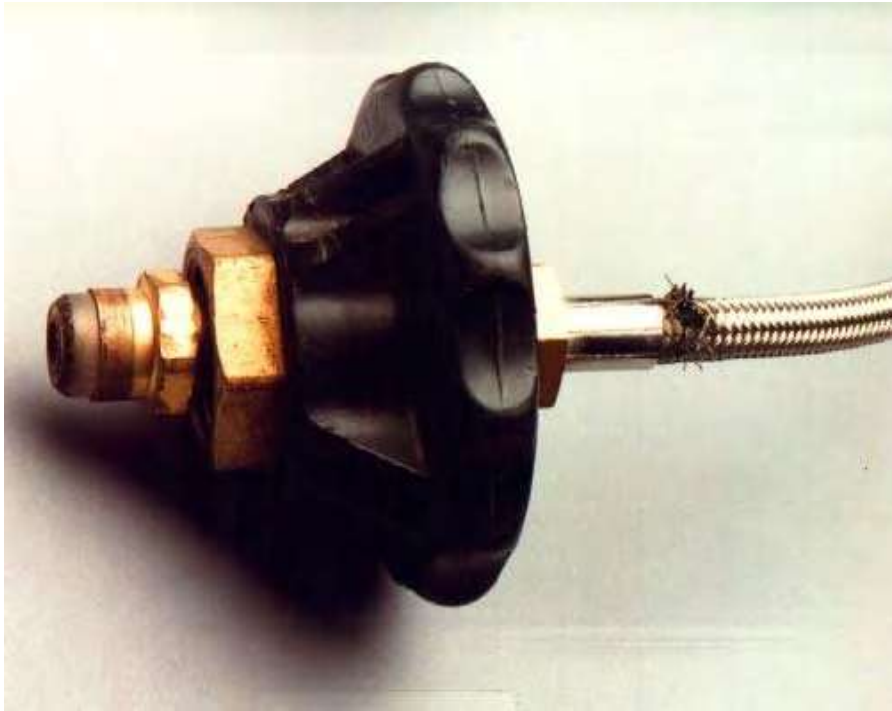
Figure 3-32-6—Burn-through of a PTFE-lined stainless steel hose in high-pressure gaseous oxygen service. Grease contamination ignited and penetrated the hose.
