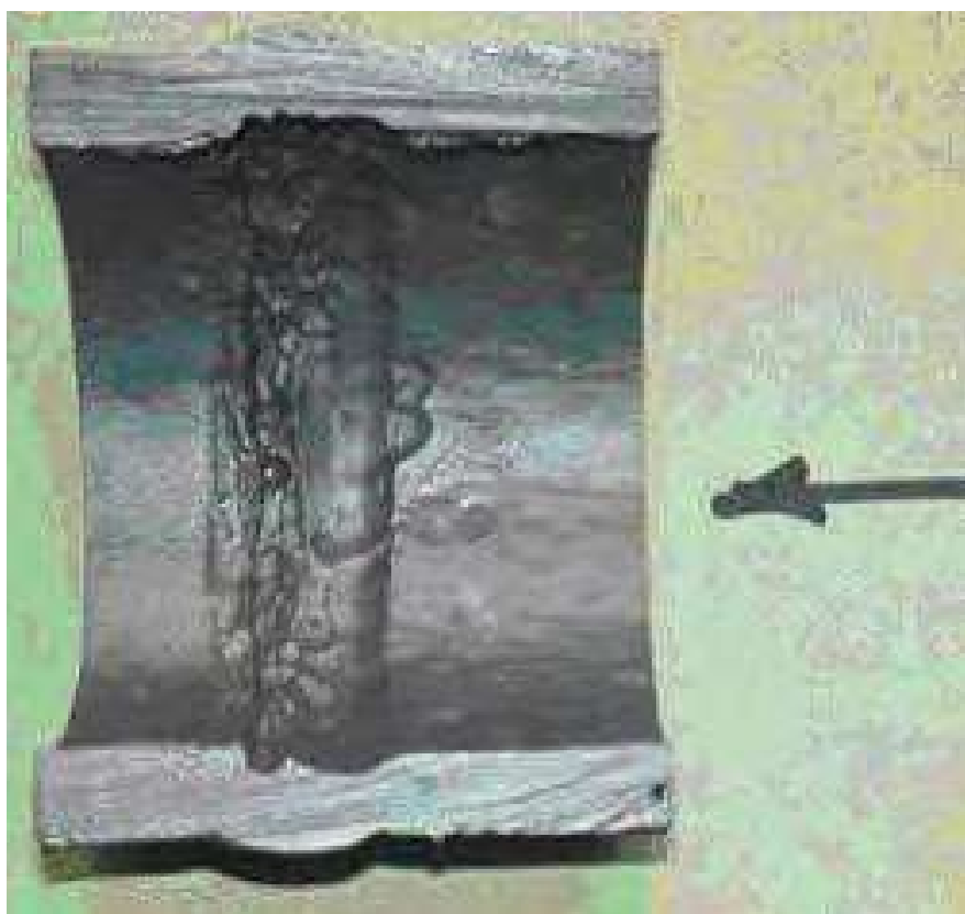
Figure 3-5-1—Ammonium bisulfide corrosion in a 2-in. CS elbow and straight section in a SW line off the cold high-pressure separator (HPS) in an HDT unit.
