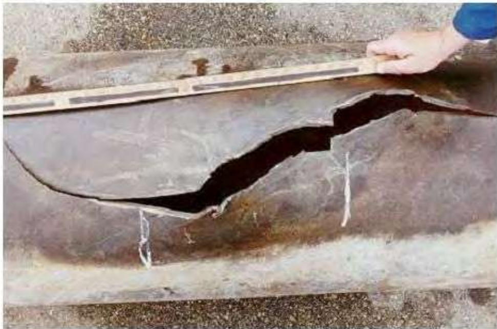
Figure 3-11-1—20-in. carbon steel pipeline that failed during hydrotest at gouges on the OD.
