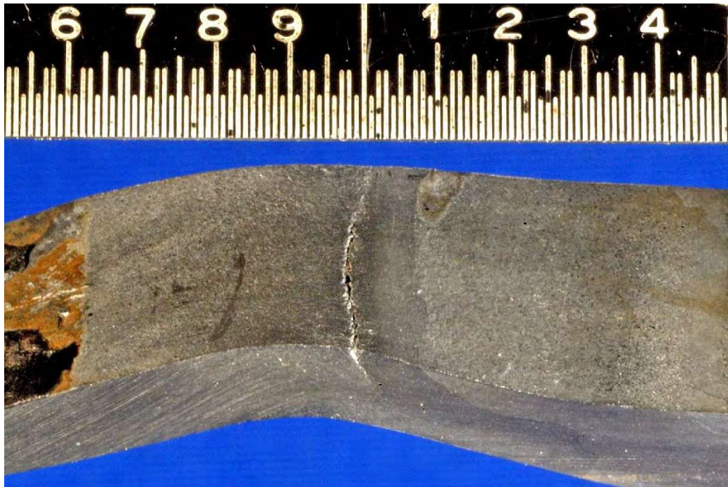
Figure 3-34-1—A crack opened up along the low-temperature edge of the HAZ when a graphitized piece of steel was subjected to a bending test. The scale in the photo is in tenths of an inch. (Reference 10)
