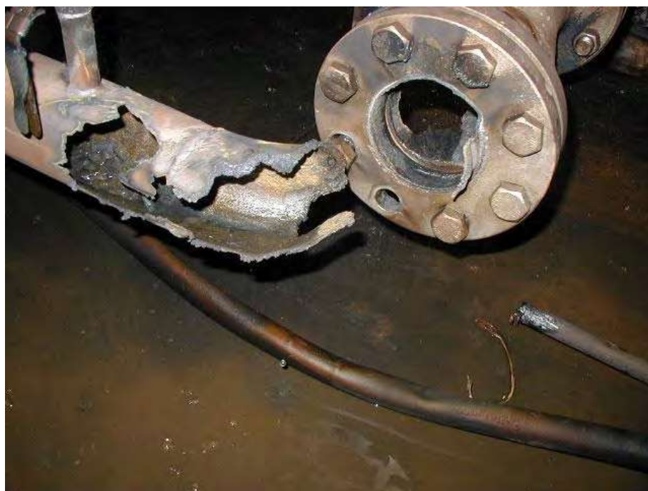
Figure 3-32-4— Photograph of a burned 304 SS elbow. The fire started in an upstream stainless steel wire filter (due to particle impact), and the burning filter material impacted the elbow and ignited it. Thin stainless steel components (e.g. filter) are much more flammable than thicker stainless steel. Thin stainless steel ( <1/8 in.) is usually avoided in oxygen systems.
