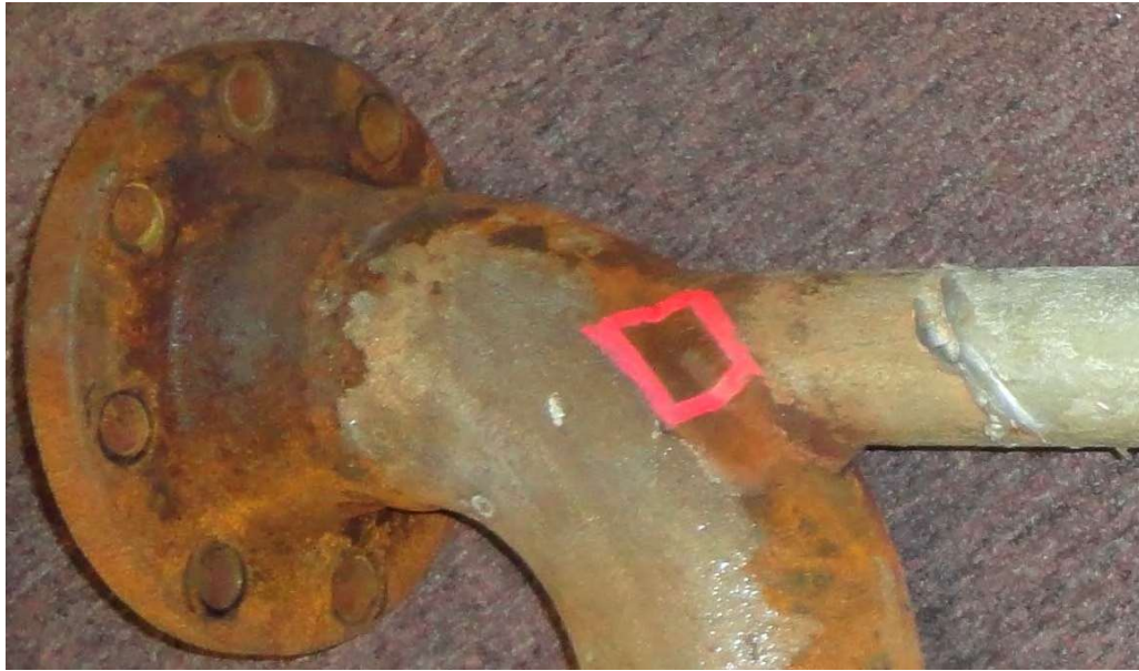
Figure 3-18-1—CO 2 corrosion caused a leak in an elbow at a support leg. The cooling effect of the support leg caused carbonic acid to condense from the vapor phase.
