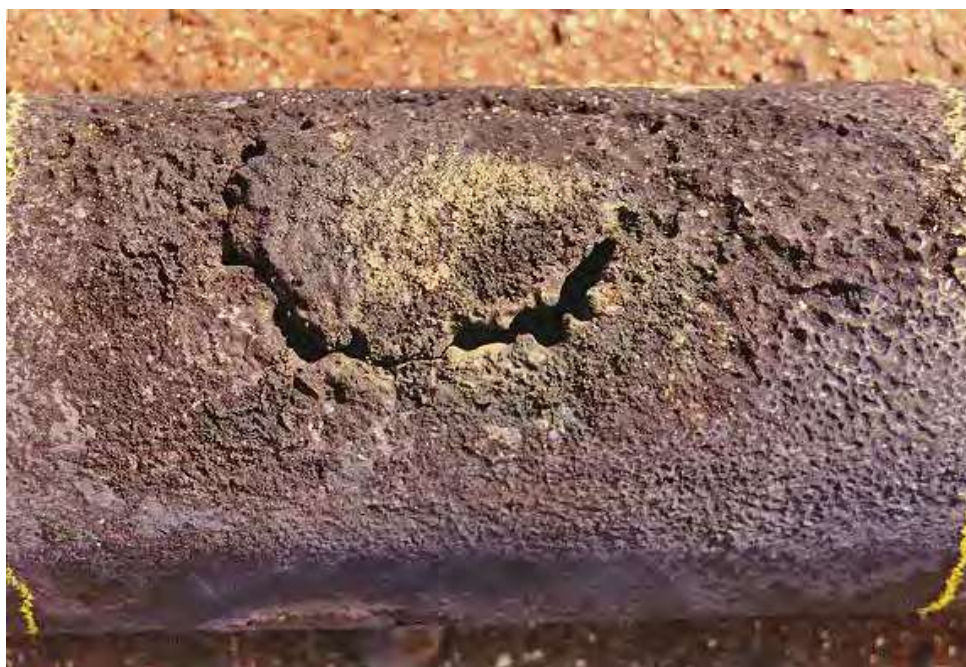
Figure 3-30-1—Type 316Ti stainless steel roof tube in a heavy fuel oil-burning vacuum heater that failed by fuel ash corrosion. The tube perforated at this location.
