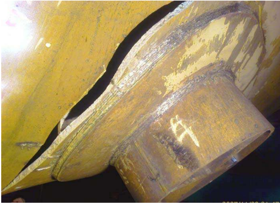
Figure 3-11-4—Brittle fracture of vessel shell during hydrotest.
