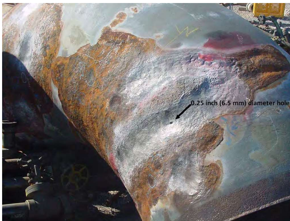
Figure 3-22-3—CUI of a 30-in. carbon steel butadiene line showing highly localized corrosion that could only be found by stripping the entire line. Note the 0.25-in. (6.5-mm) diameter hole at arrow.
