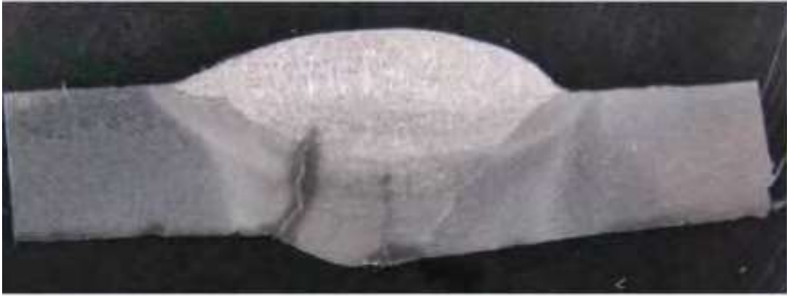
Figure 3-12-6—Most cracks originate in base metal, but this weldment contained a crack that originated at the root and propagated through the weld metal. Other cracks appear to have initiated in the HAZ. (Reference 7)
