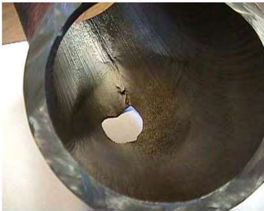
Figure 3-27-2—Erosion of a 9Cr-1Mo coker heater return bend as the result of high steam-air decoking velocity.
