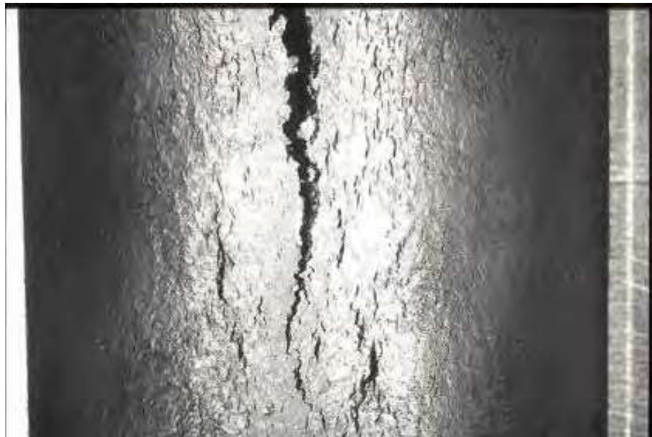
Figure 3-23-2—Creep rupture of an HK40 heater tube.
