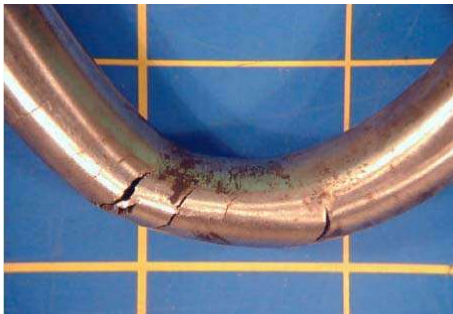
Figure 3-17-1—External cracking of Type 304 SS instrument tubing under insulation.
