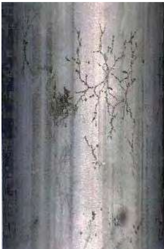
Figure 3-17-3—Cracking on the shell side of a Type 316L SS tube in steam service at 450 °F (230 °C) showing tight cracks with a crazed or spider web appearance.
