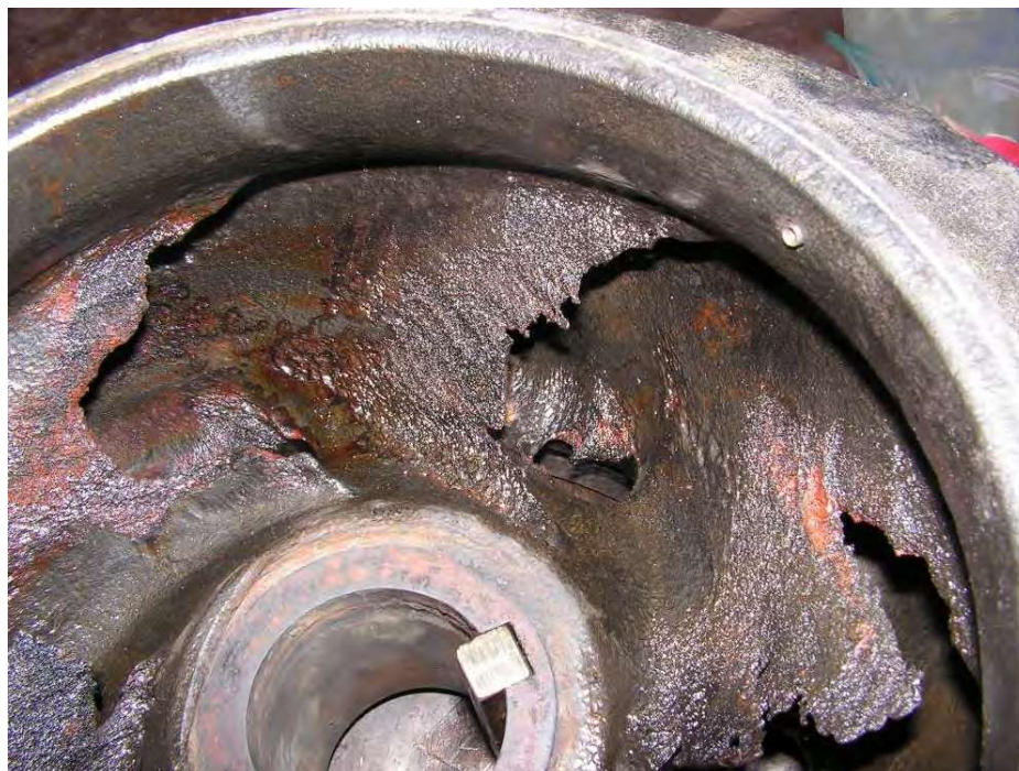
Figure 3-27-3—Erosion-corrosion of an ASTM A48 Class 30 cast iron impeller in a recycle water pump.
