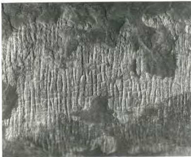
Figure 3-30-4—The “alligator hide” morphology of liquid coal-ash corrosion is evident on the metal surface when the dense, glassy deposit is removed. Magnification 2.4X.
