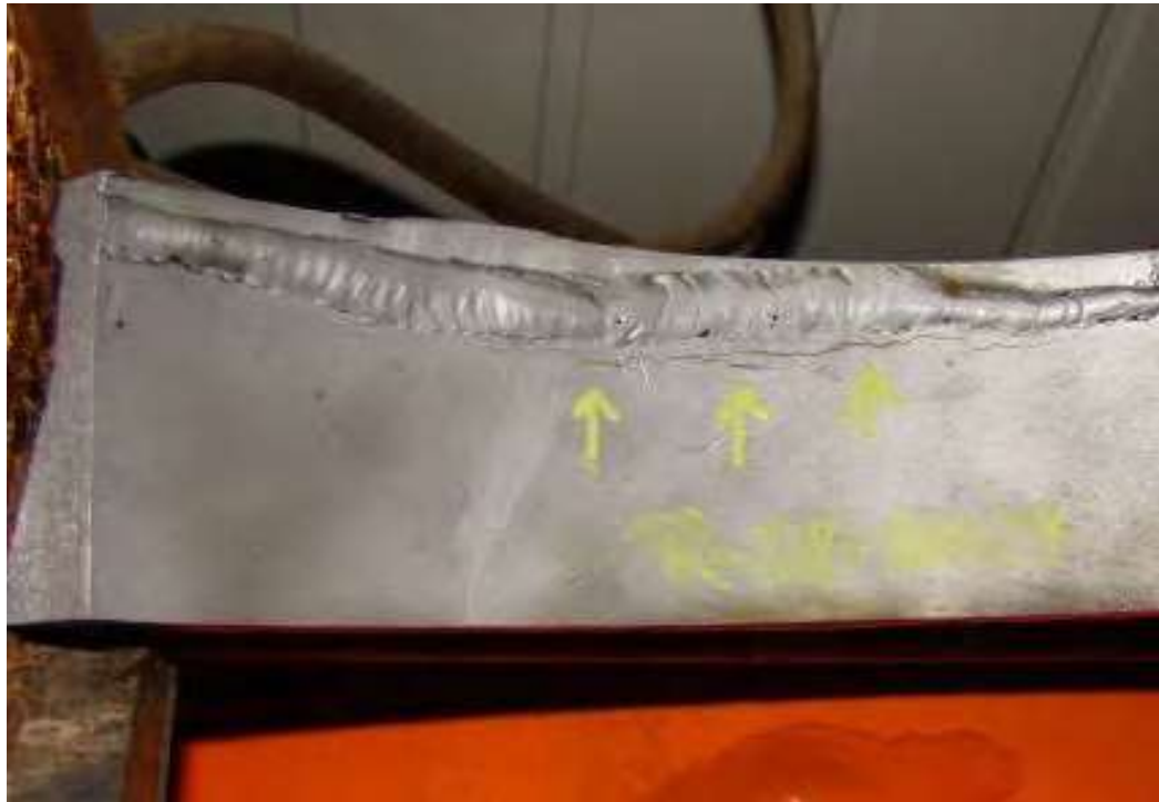
Figure 3-12-3—Carbonate cracking in an overhead interstage knockout drum vapor outlet nozzle.
