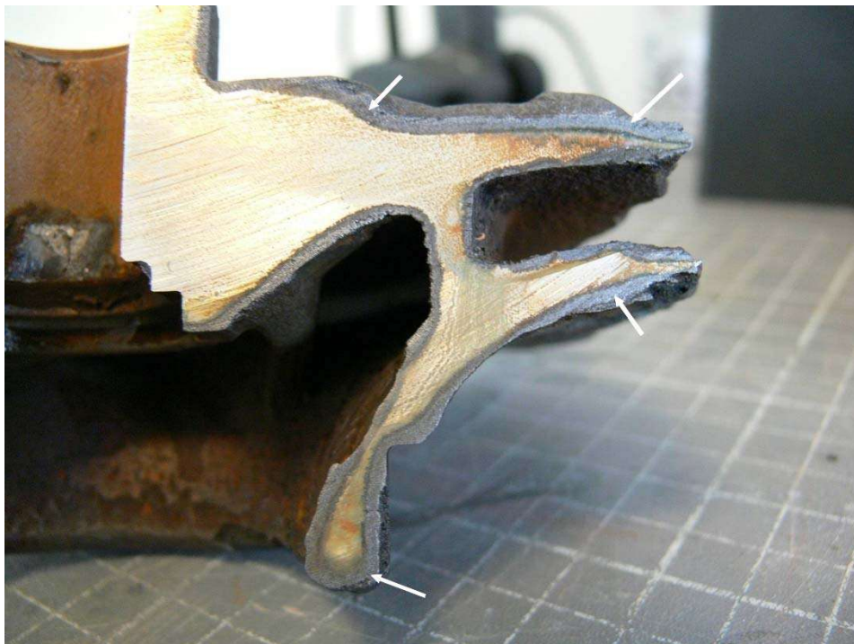
Figure 3-33-2—Cutaway of the cast iron impeller shown in Figure 3-32-1. The dark phase around the outside perimeter (at arrows) is graphite that surrounds the unaffected metal in the middle.
