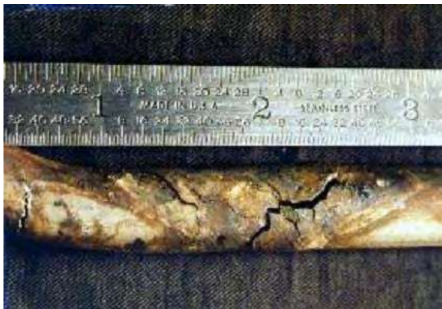
Figure 3-17-2—External cracking of Type 304 SS instrument tubing under insulation.
