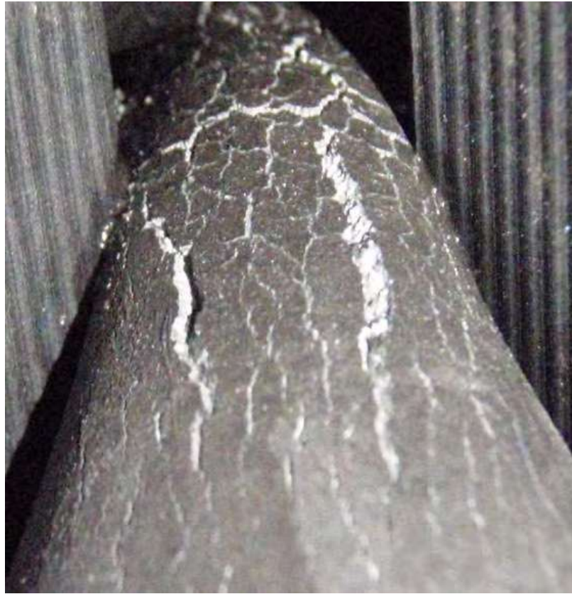
Figure 3-23-1—A pinched Alloy 800H pigtail with opened-up creep fissures on the surface.
