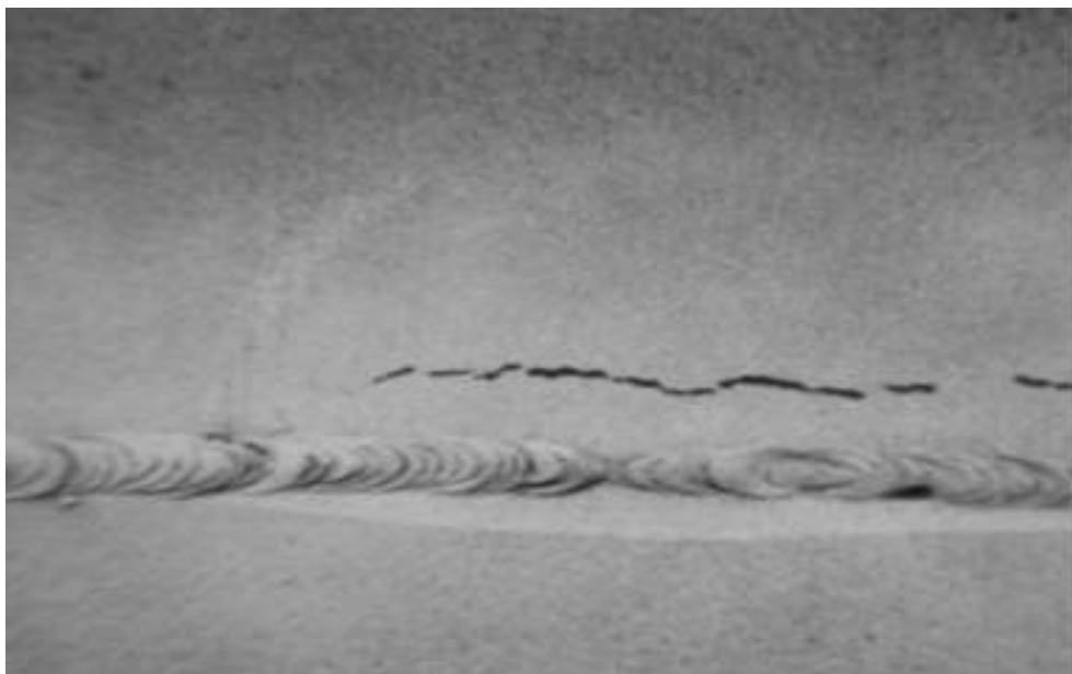
Figure 3-12-4—Carbonate cracking adjacent to a weld. (Reference 6)
