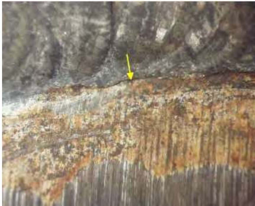
Figure 3-26-4—Weld detail used to join a carbon steel elbow (bottom) to a weld overlaid pipe section (top) in high-pressure wet H 2 S service. SSC occurred along the toe of the weld (arrow), in a narrow zone of high hardness.
