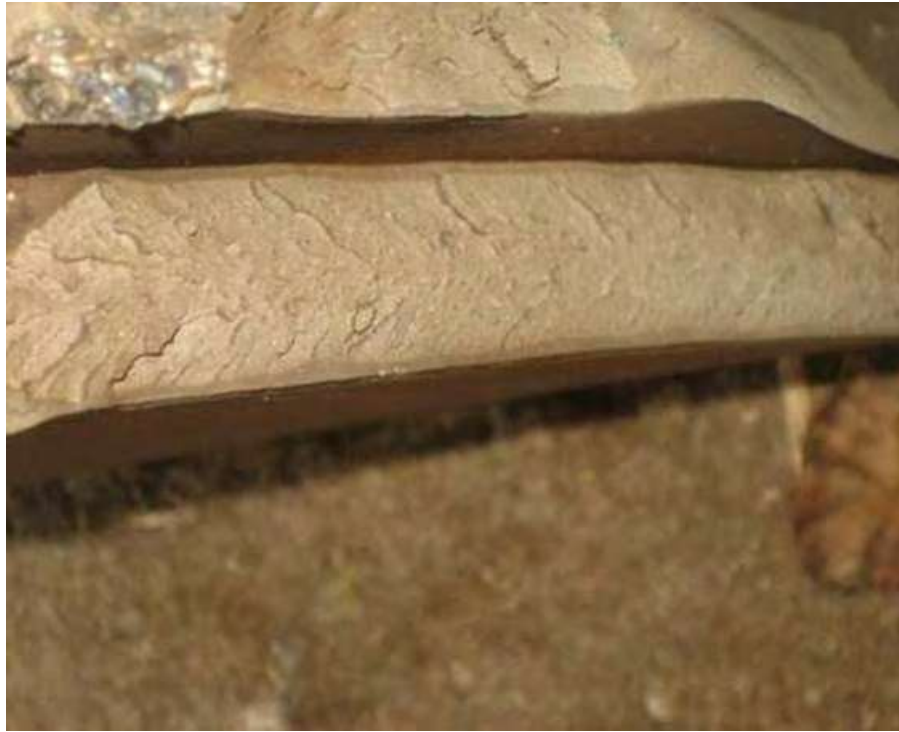
Figure 3-11-6—Close-up view of the fracture surface from a vessel made of A516-70N plate showing the chevron pattern that points back toward the origin of the crack.
