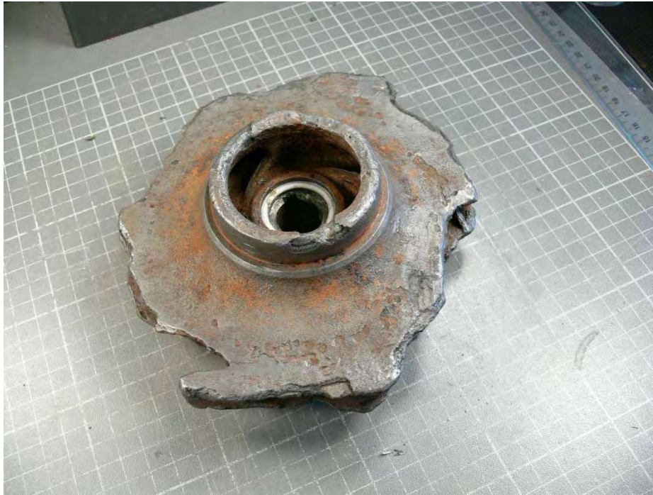
Figure 3-33-1—Graphitic corrosion of a cast iron pump impeller due to glycol acidification.
