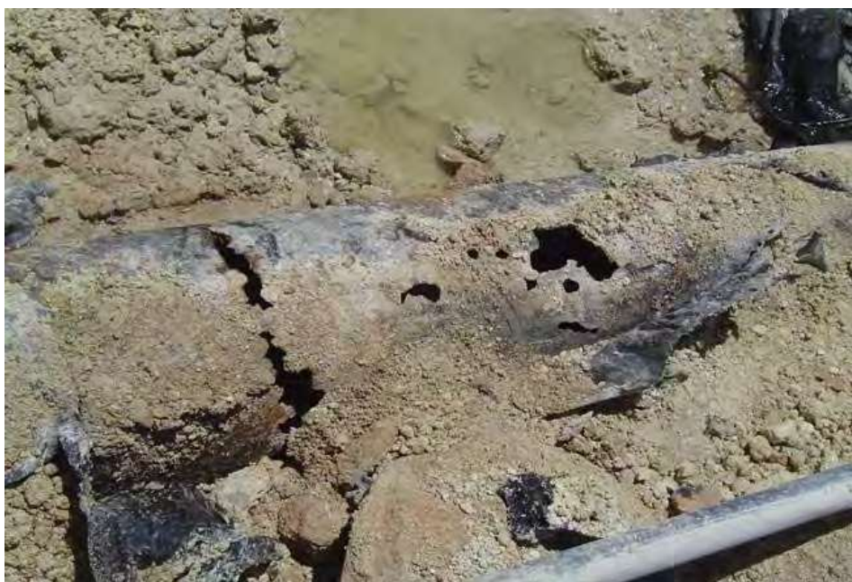
Figure 3-33-3—View of the outside of an underground concrete-lined saltwater service line that failed from graphitic corrosion.
