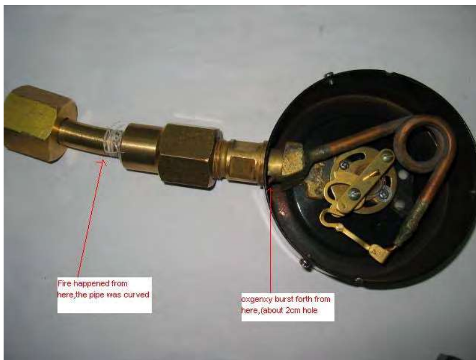
Figure 3-32-5— Photograph illustrating burn-through of a brass pressure gage. Brass is generally suitable for oxygen service. However, the gauge was not intended for oxygen service and was not “oil free.” Hydrocarbon contamination, probably from manufacture, caused the fire.
