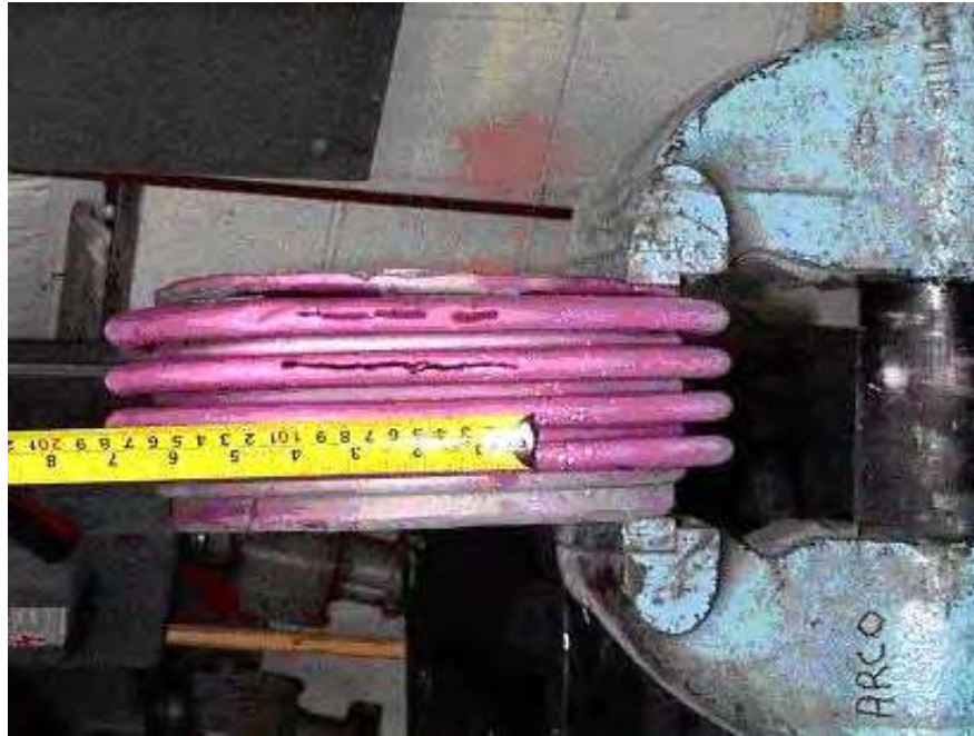
Figure 3-15-8—Stainless steel expansion bellows from a steam-driven turbine previously subjected to a caustic carryover upset condition.
