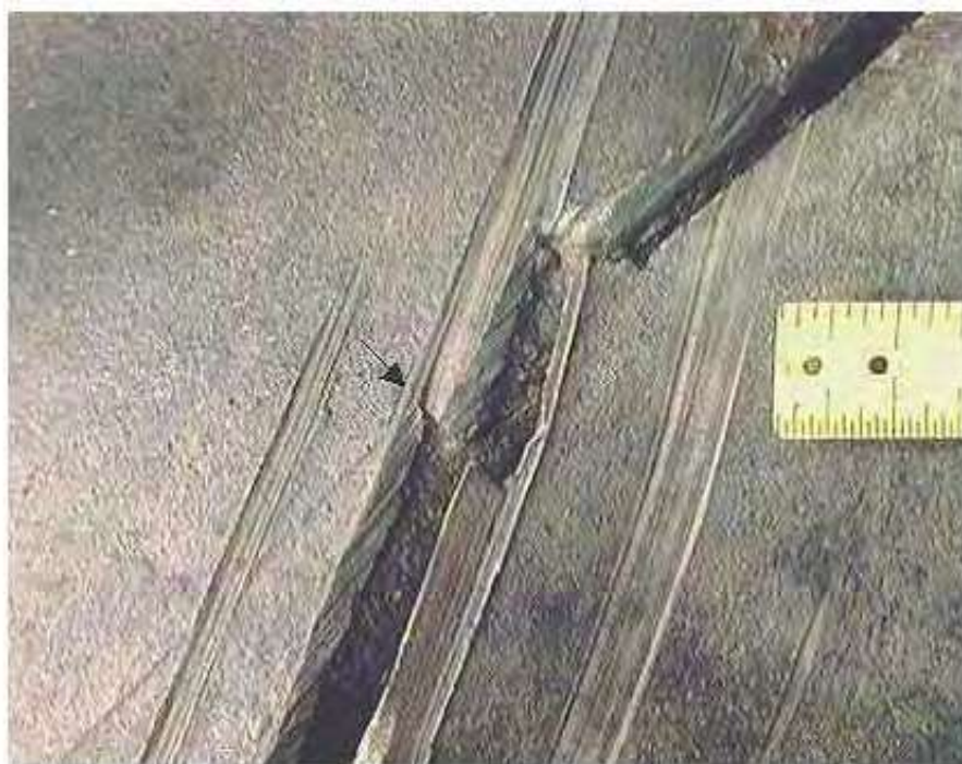
Figure 3-11-2—Close-up of Figure 3-11-1 showing the gouges and the fracture origin (arrow) in one of the gouges.
