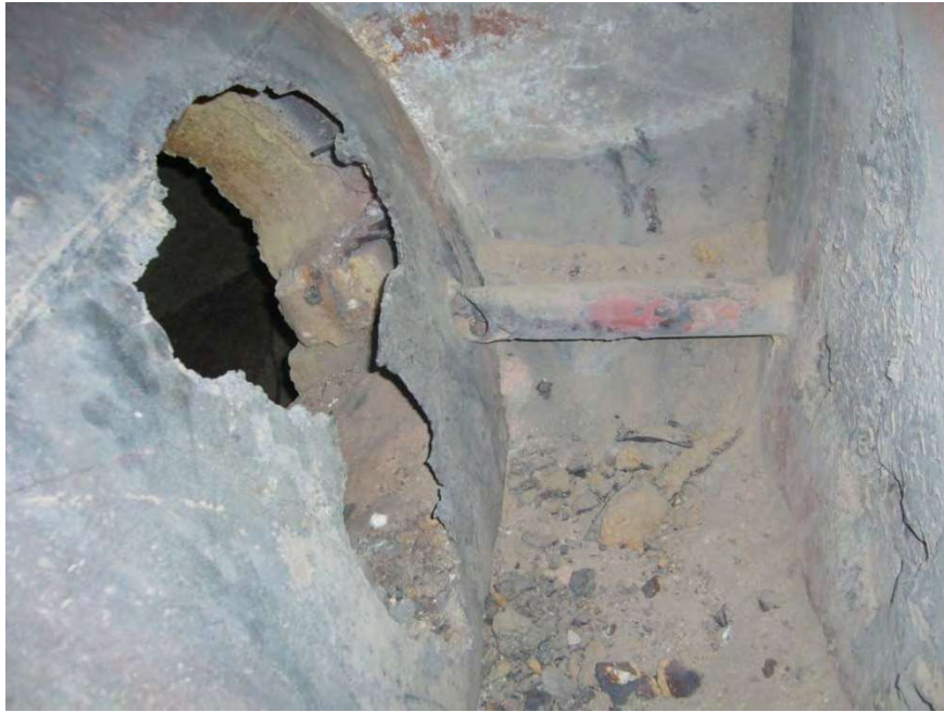
Figure 3-32-2—Same as figure above after damage due to oxygen combustion resulting from oxygen injection into the thermal combustor on the front end of the reaction furnace.
