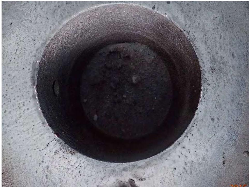
Figure 3-3-2—Radial amine SCC cracks emanating from the bore of a nozzle in a rich amine reboiler exchanger.
