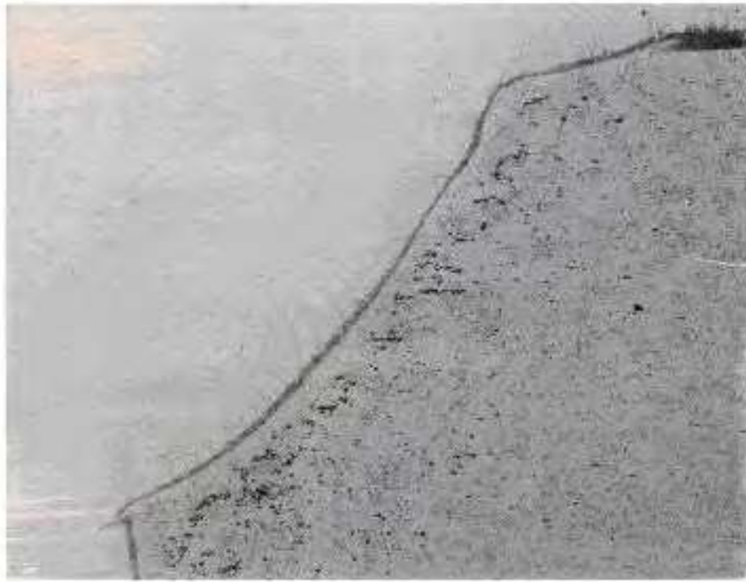
Figure 3-26-3—High-magnification photomicrograph of a DMW joining a ferritic alloy (SA213 T-22) used in high-temperature service. Creep cracks (black specks) can be observed in the ferritic alloy HAZs. Magnification 50X, etched.
