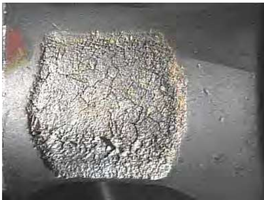
Figure 3-24-2—A zone of denickelification in an Alloy 400 valve plug (at the port), due to oxygen contamination in hot hydrofluoric acid.
