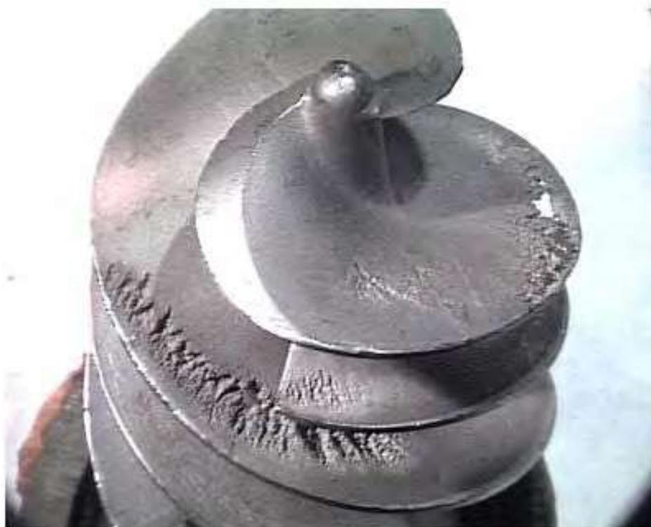
Figure 3-16-4—Cavitation pitting on the low-pressure side of a stainless steel pump impeller.
