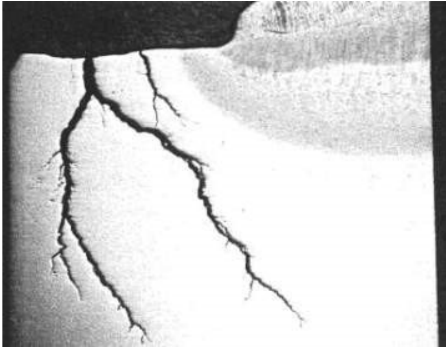
Figure 3-3-1—A photomicrograph of a cross section of a weld in non-PWHT'd carbon steel piping showing amine SCC in the vicinity of a piping weld. Magnification 6X (from API 945).
