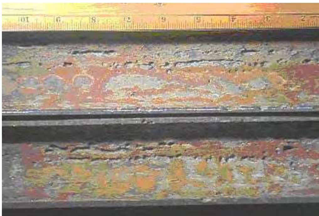
Figure 3-18-3—CO 2 corrosion of a carbon steel oil and gas production flow line.
