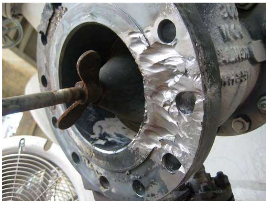
Figure 3-27-1—Erosion-corrosion of a 1¼Cr-½Mo, 300-lb valve flange on an FCC catalyst withdrawal line.
