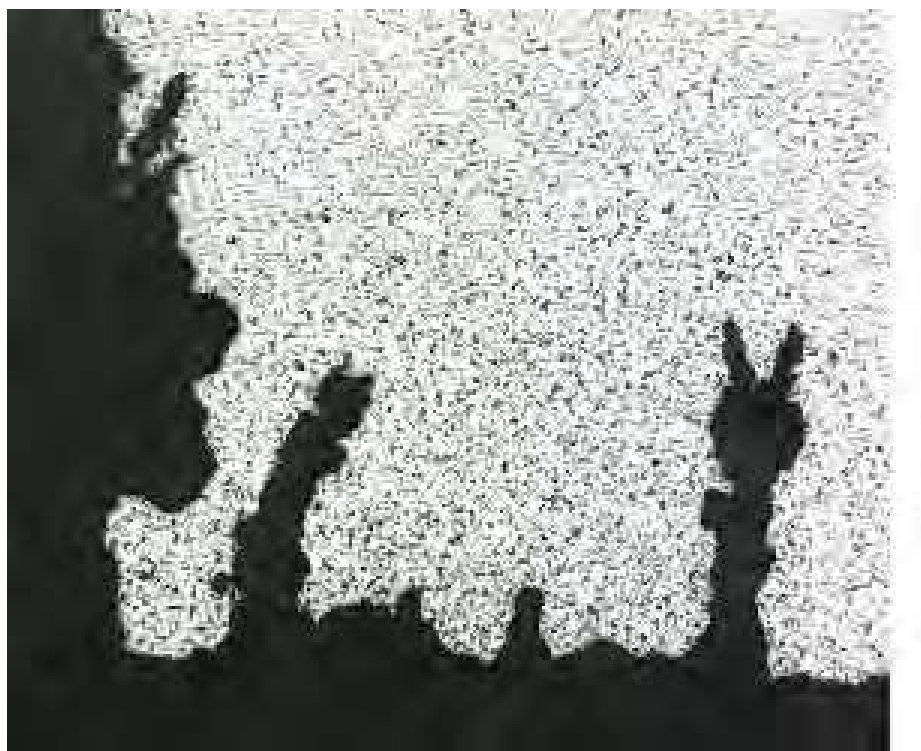
Figure 3-21-5—Photomicrograph showing the crack morphology that is rounded with multiple lobes and may branch to form “rabbit ears.” (Magnification 25X, etched.)
