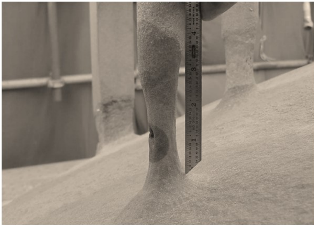
Figure 3-22-5—CUI of a nozzle on the top head of a pressure vessel.
