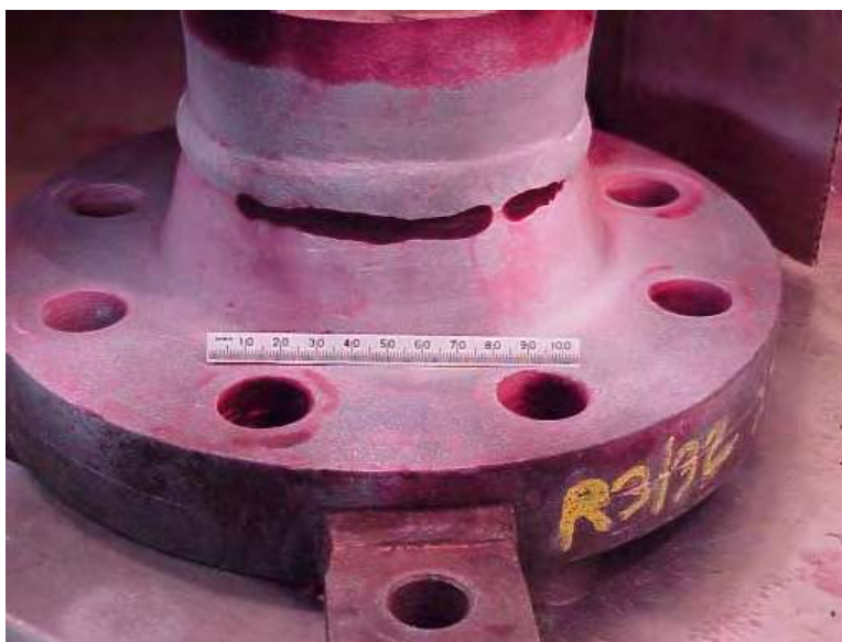
Figure 3-26-9—Failure of nickel alloy DMW joining HP40 (Nb-modified) tube to 1.25Cr-0.5Mo flange in a steam-methane reformer due to cold hydrogen disbonding of the buttering layer. Process temperature 915 °F to 940 °F (490 °C to 505 °C), pressure 310 psig (2.15 MPa), H 2 content 10 % to 20 % (off-gas).
