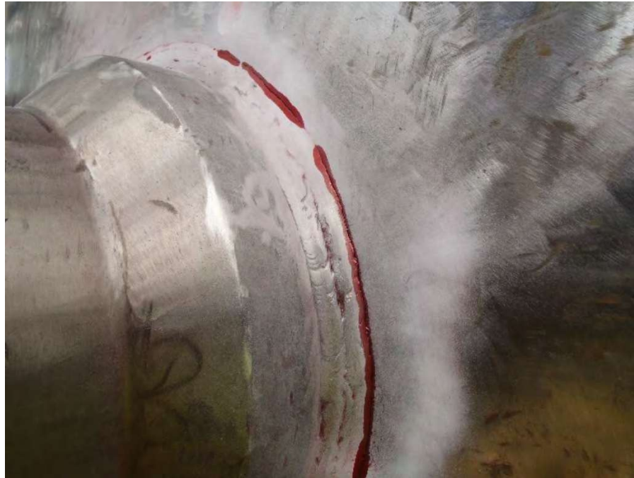
Figure 3-26-11—A crack around the base of an Alloy 400 nozzle welded into a carbon steel vessel in HF acid service. (Reference 15)
