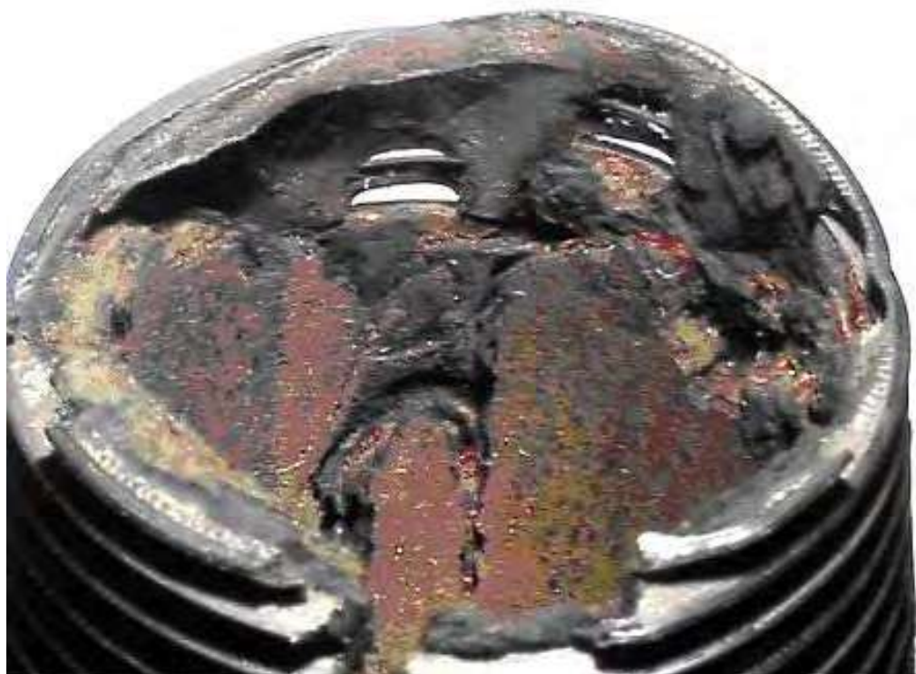
Figure 3-18-5—CO 2 corrosion of a carbon steel pipe nipple in CO 2 -contaminated water.
