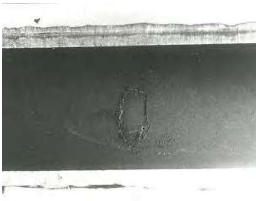
Figure 3-21-4—Photograph of a carbon steel boiler tube cut in half lengthwise. Corrosion fatigue cracks initiated at the ID of the tube, opposite a buckstay attachment on the OD. (Magnification 1X.)
