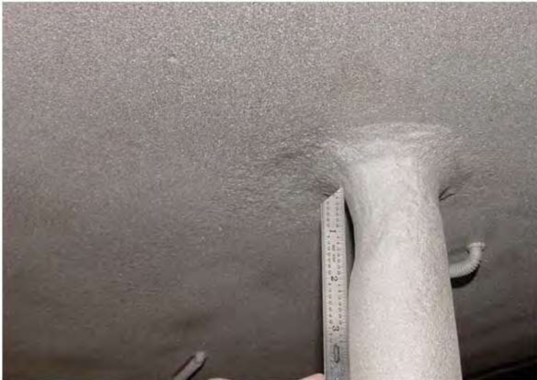
Figure 3-22-4—CUI of a nozzle on the bottom head of a pressure vessel.
