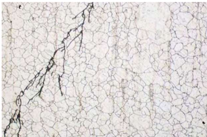
Figure 3-15-10—Micrograph showing transgranular caustic SCC in Alloy 825. Magnification 200X. (Reference 5)
