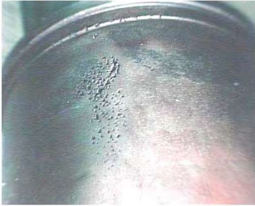
Figure 3-16-5—Pitting caused by cavitation on the water side of a cast iron cylinder liner in a large engine.
