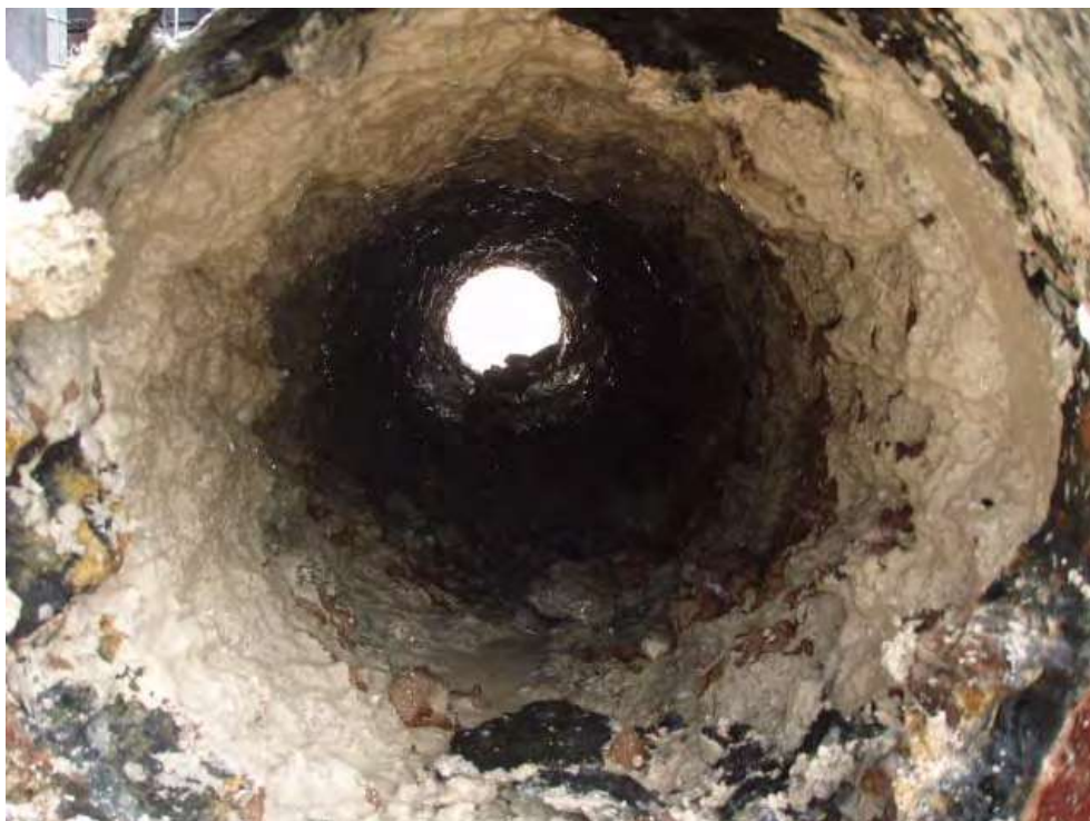
Figure 3-33-4—View of concrete lining inside the failed line shown in Figure 3-32-3.
