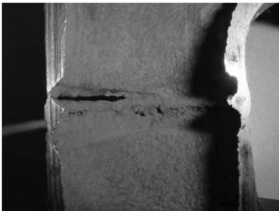
Figure 3-38-6—Accelerated corrosion in the HAZ of a carbon steel weldment. RE content is as follows. (Reference 8) Both base metals: %C > 0.18 wt %; %Cu + %Ni < 0.15. Weld metal: %Cu + %Ni + %Cr < 0.15.
