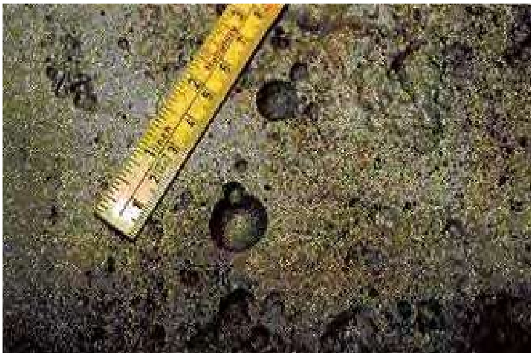
Figure 3-45-5—Same oil line as Figure 3-43-4. Hemispherical pitting typical of MIC can be seen after grit blasting to remove the scale.
