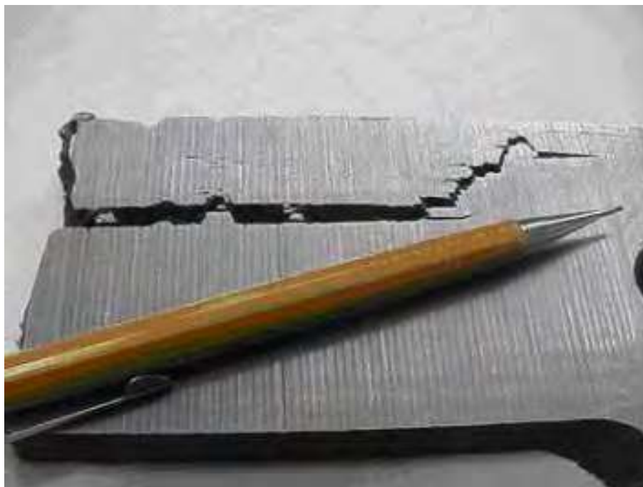
Figure 3-67-3—HIC damage as shown in the cross section of the shell of a trim cooler that had been cooling vapors off a hot high-pressure separator (HHPS) vessel in a hydroprocessing unit.
