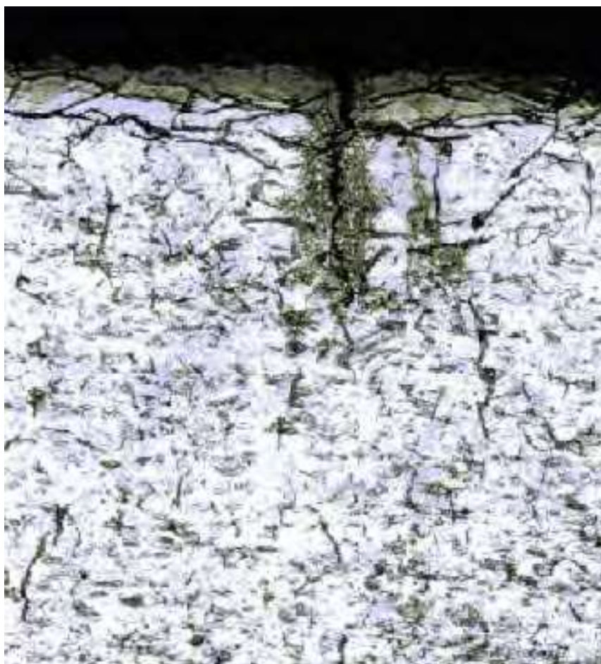
Figure 3-66-2—High-magnification photomicrograph of a cross section of the tube shown in Figure 3-66-1 through the crack tip. Magnification 200X.
