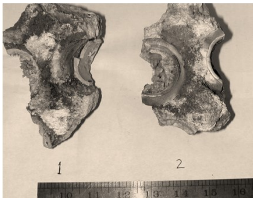
Figure 3-53-1—Damaged refractory and ferrules.
