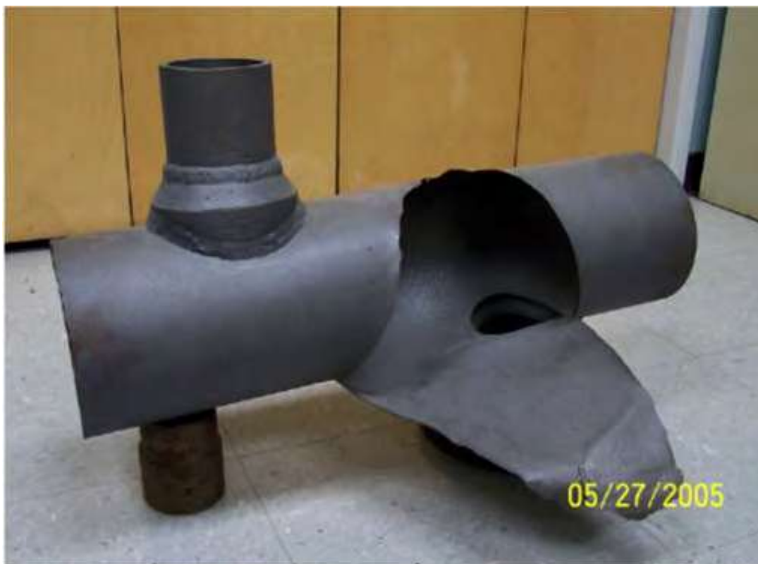
Figure 3-61-3—Sulfidation failure of an 8-in. carbon steel pipe. Note the relatively uniform thinning that resulted in a sizeable rupture.
