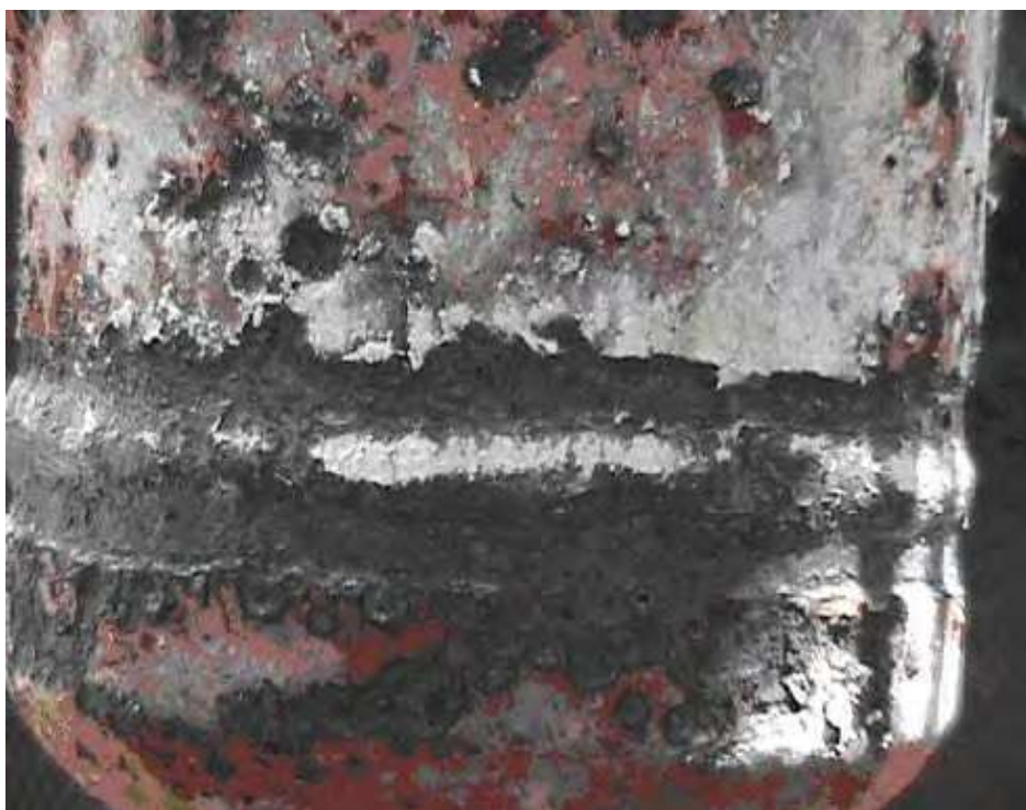
Figure 3-48-4—Oxidation of the OD of a carbon steel furnace transfer line.
