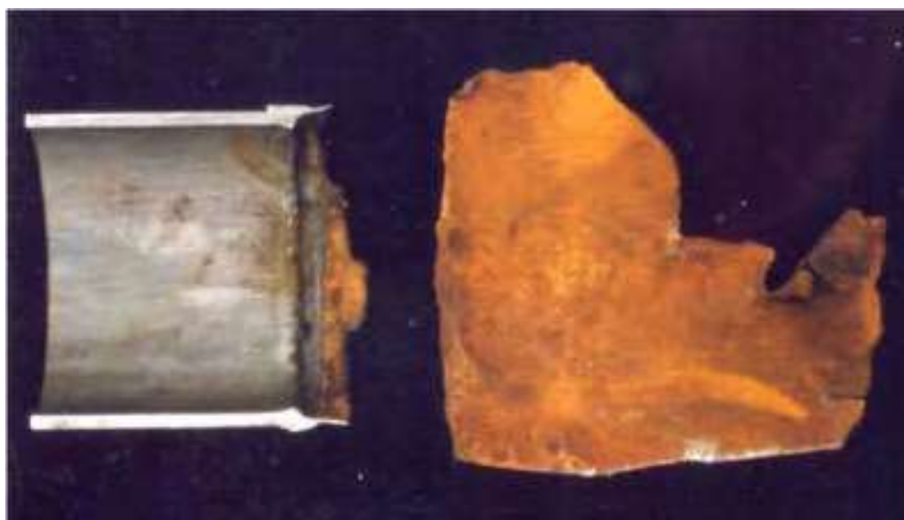
Figure 3-38-4—Ruptured NPS 3 Sch. 80 [0.216 in. (5.5 mm) wall thickness] depropanizer feed line operating < 120 °F (50 °C). RE content is as follows. Both base metals: %C > 0.18 wt %; %Cu + %Ni < 0.15. Weld metal: %Cu + %Ni + %Cr < 0.15.
