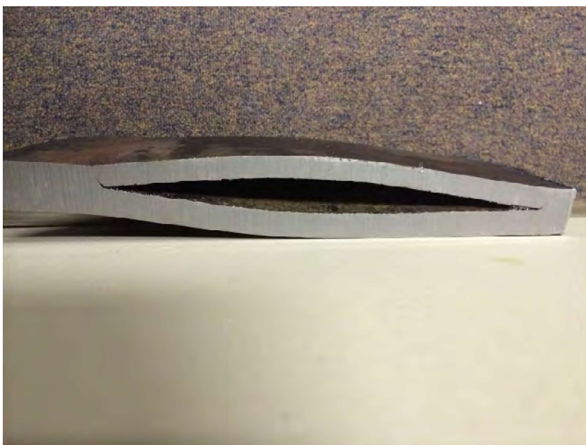
Figure 3-38-8—Internal blister caused by HF corrosion near the top of a 1.2-in.-thick carbon steel tower in an HF alkylation unit. The maximum measured dimensions of the blister were 2 ft high and 20 ft long (circumferentially). The hanging weight of an adjacent tray, which was also badly corroding, may have contributed to the location and size of the blister.
