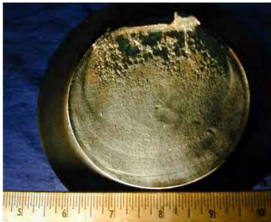
Figure 3-43-6—Compressor rod fracture surface showing “beach marks.”
