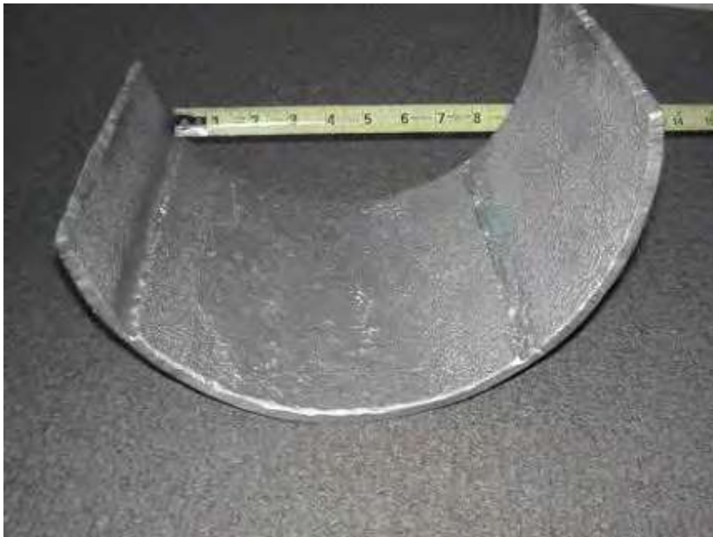
Figure 3-62-3—Grooving corrosion in the carbon steel vapor line from an alkaline water wash drum in a sulfuric acid alkylation unit.
