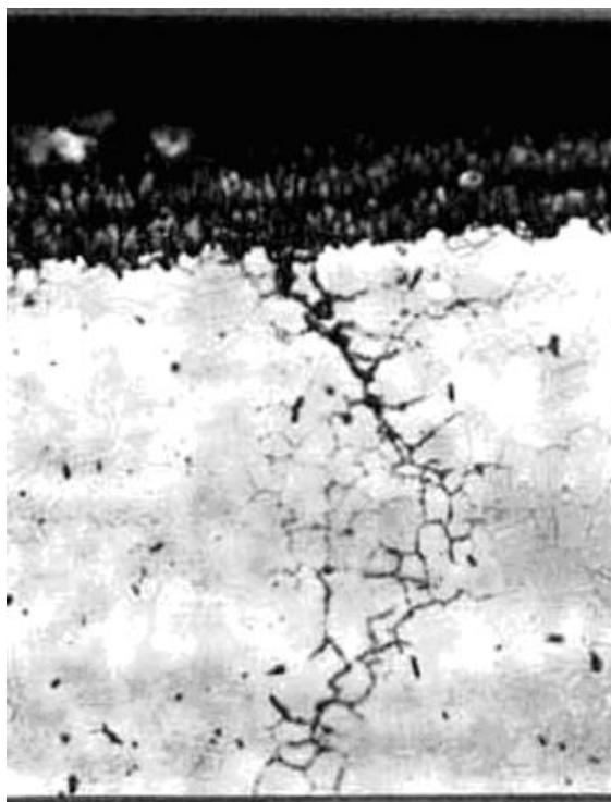
Figure 3-42-2—Photomicrograph of a section of the elbow in Figure 3-40-1, illustrating the intergranular nature of zinc-filled cracks in stainless steel.
