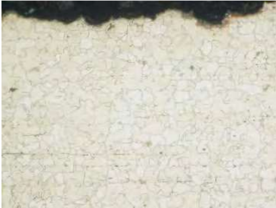
Figure 3-36-4—A photomicrograph at the ID surface of the pipe in Figure 3-35-2 shows complete decarburization of the original structure. Magnification 200X.
