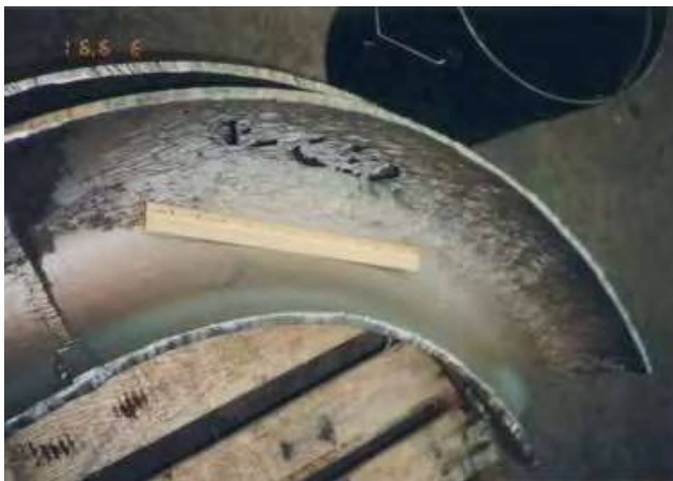
Figure 3-46-1—Erosion-corrosion damage due to NAC in a 10-in. 5Cr- \frac{1}{2} Mo elbow in the outlet of a vacuum heater in a vacuum distillation unit.
