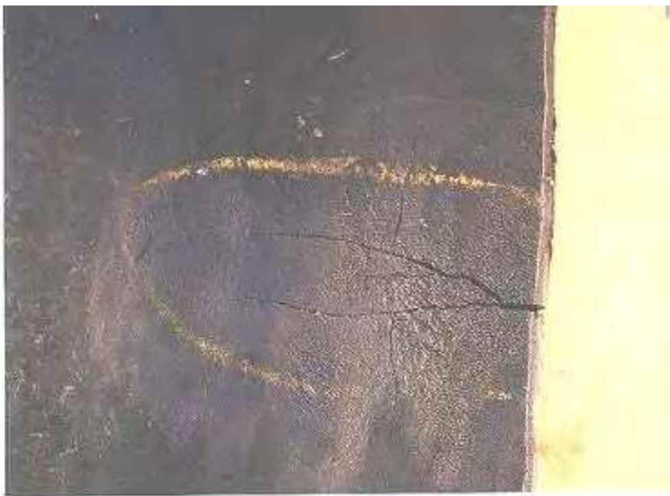
Figure 3-42-3—LME of Monel caused by mercury in an FCC gas plant overhead drum.
