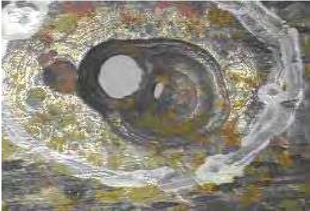
Figure 3-45-2—Pitting corrosion on the ID of a 6-in. carbon steel sour crude line after 2½ years of service. Pits are approximately 1-in. to 2-in. wide. Note the halo effect in Figure 3-43-3.
