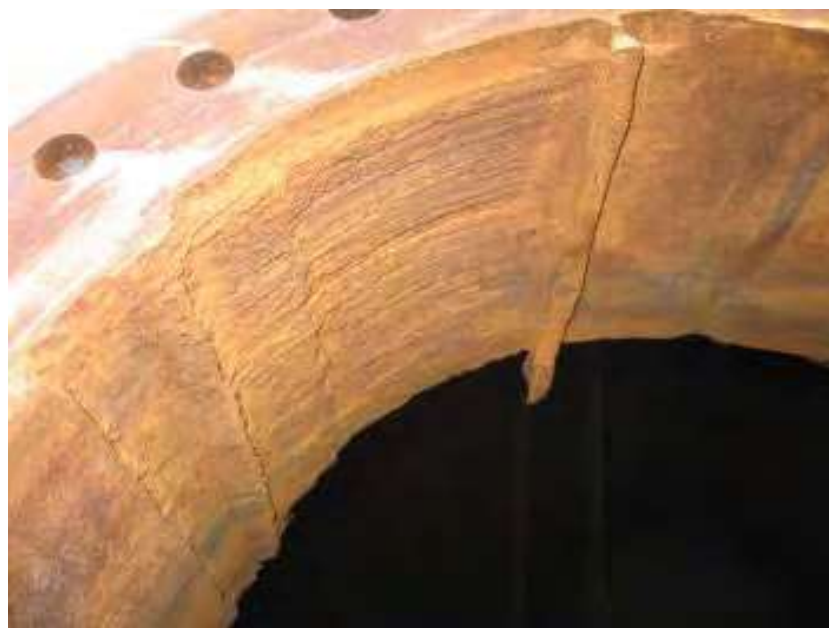
Figure 3-38-7—HF corrosion at a manway in HF acid storage service.
