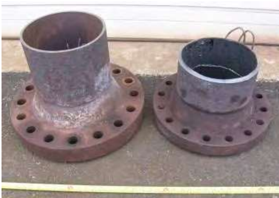
Figure 3-36-2—A pair of 10-in. C- \frac{1}{2} Mo flanged pipe sections (SA335-P1 and SA234-WP1) from a hot bypass line in a catalytic reformer that was designed to remain closed but operated partially or fully open for unknown lengths of time. They were in service for ~34 years at temperatures up to 960 °F (515 °C) with a hydrogen partial pressure of 198 psig (1.4 MPa).
