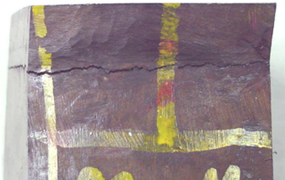
Figure 3-54-2—Crack at weld from Type 321 SS elbow shown in Figure 3-52-1.
