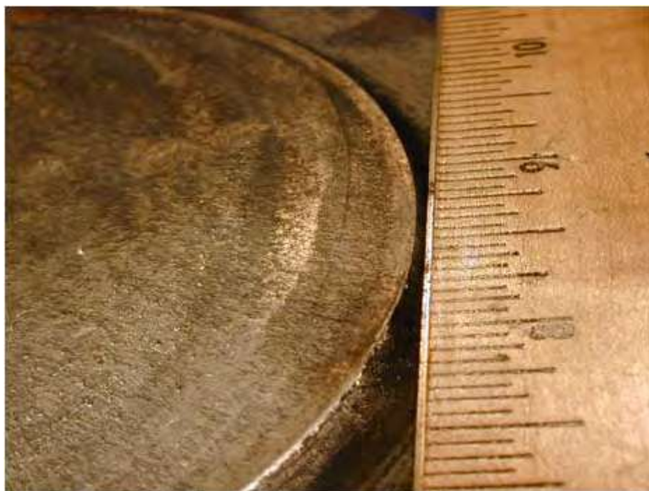
Figure 3-43-7—Higher-magnification view of Figure 3-41-6 above showing “beach marks.”
