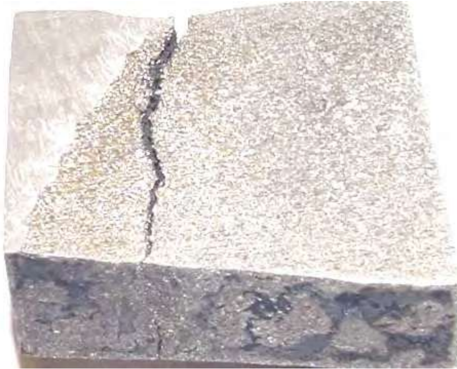
Figure 3-54-3—Cross section through the weldment showing the crack in Figure 3-52-2.
