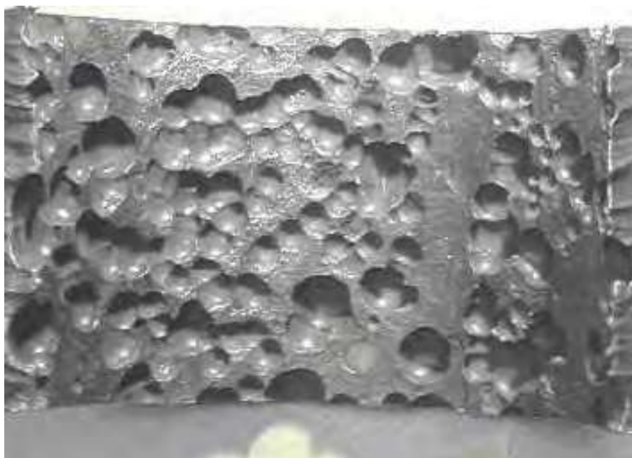
Figure 3-44-1—Metal dusting of a 304H stainless steel pipe.
