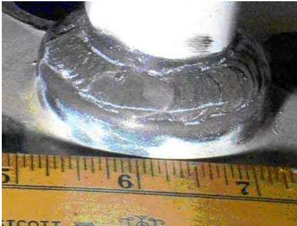
Figure 3-43-1—Vibration induced fatigue of a 1-in. socket weld flange in a thermal relief system shortly after start-up.
