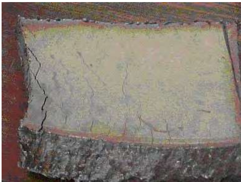
Figure 3-64-1—Thermal fatigue cracks on the inside of a heavy wall SS pipe downstream of cooler H 2 injection into a hot hydrocarbon line.
