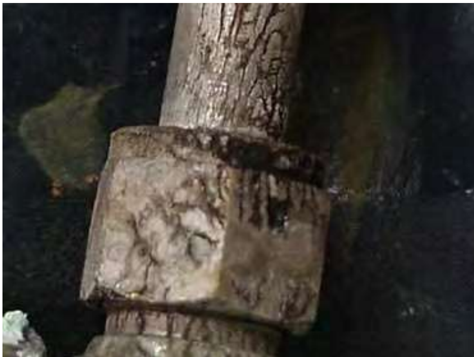
Figure 3-39-2—HF SCC of Alloy 400 instrument tubing. (Reference 7)
