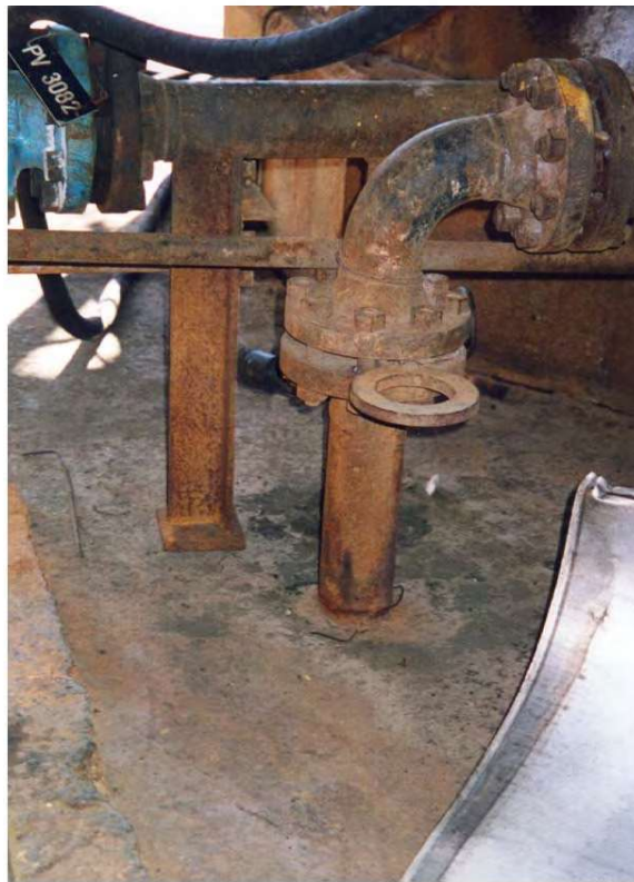
Figure 3-57-1—Corrosion of carbon steel pipe at the soil/air interface where the pipe emerges from underground.
