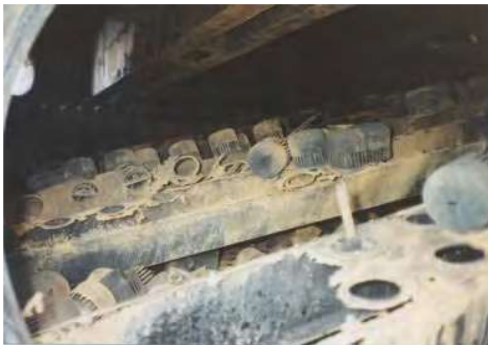
Figure 3-46-2—Severe NAC of 410 SS trays and bubble caps in the HVGO section of the vacuum tower fed by the vacuum heater referred to in Figure 3-44-1.
