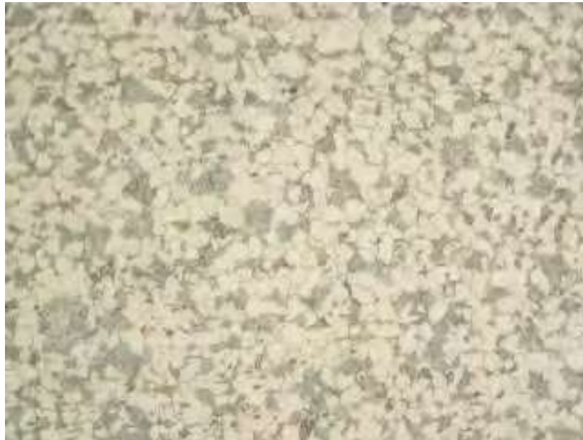
Figure 3-36-3—A photomicrograph of the OD surface of a pipe section from Figure 3-35-2 exhibits a normal ferritic-pearlitic microstructure. Magnification 200X.
