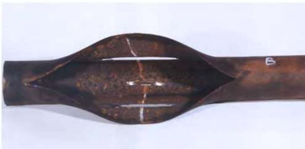
Figure 3-55-2—Tube bulged and ruptured due to short-term overheating at a temperature well over 1380 °F (750 °C).
