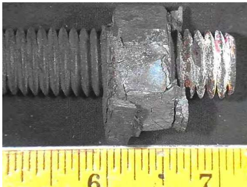
Figure 3-48-2—Oxidation of a carbon steel nut on a stainless steel stud at 1300 °F (705 °C).
