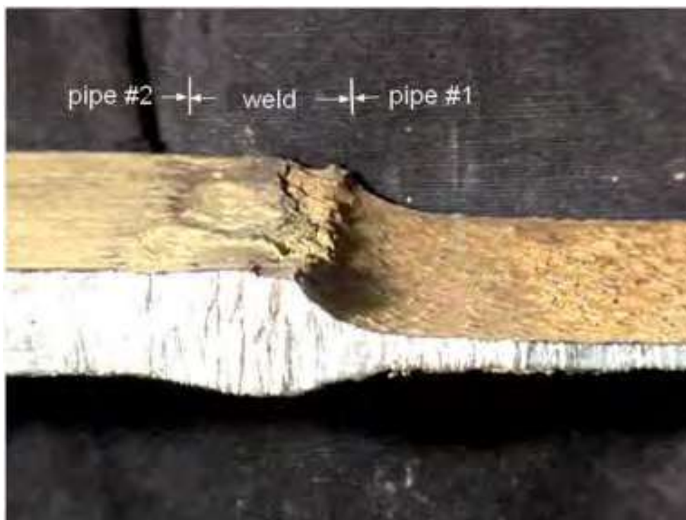
Figure 3-38-3—Cross section of a carbon steel pipe showing preferential corrosion of the pipe with high RE content on the right, as compared to the low-RE pipe section to the left of the weld. (Reference 3)
