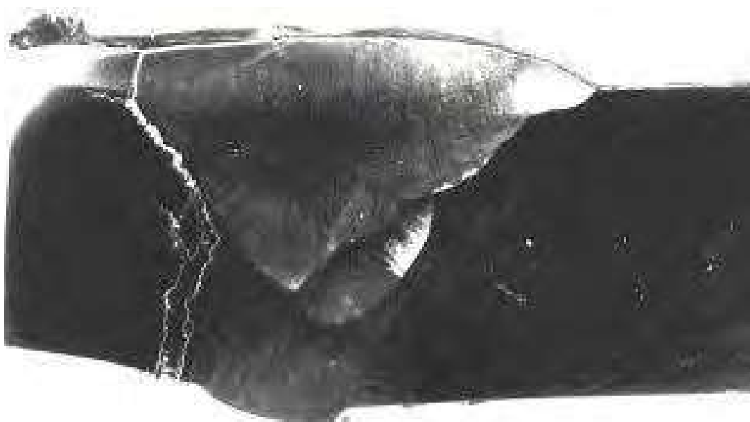
Figure 3-52-4—Cross section of the catalyst withdrawal line attached to the flange in Figure 3-50-3 showing cracking in the weld HAZ. Magnification 3X.
