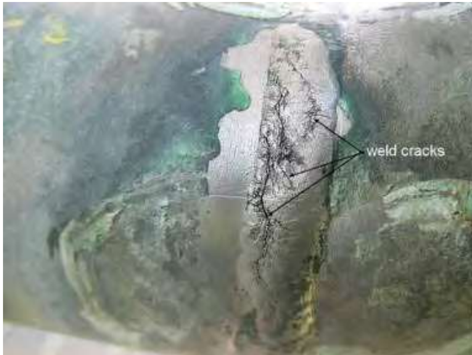
Figure 3-39-1—HF SCC of an Alloy 400 vent line in an acid dump system. (Reference 7)
