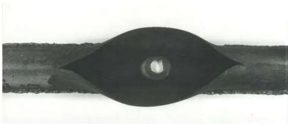
Figure 3-55-5—Short-term, high-temperature boiler tube failures from DNB are wide-open bursts with the failure lips drawn to a near knife edge. They are ductile ruptures. Magnification 25X.
