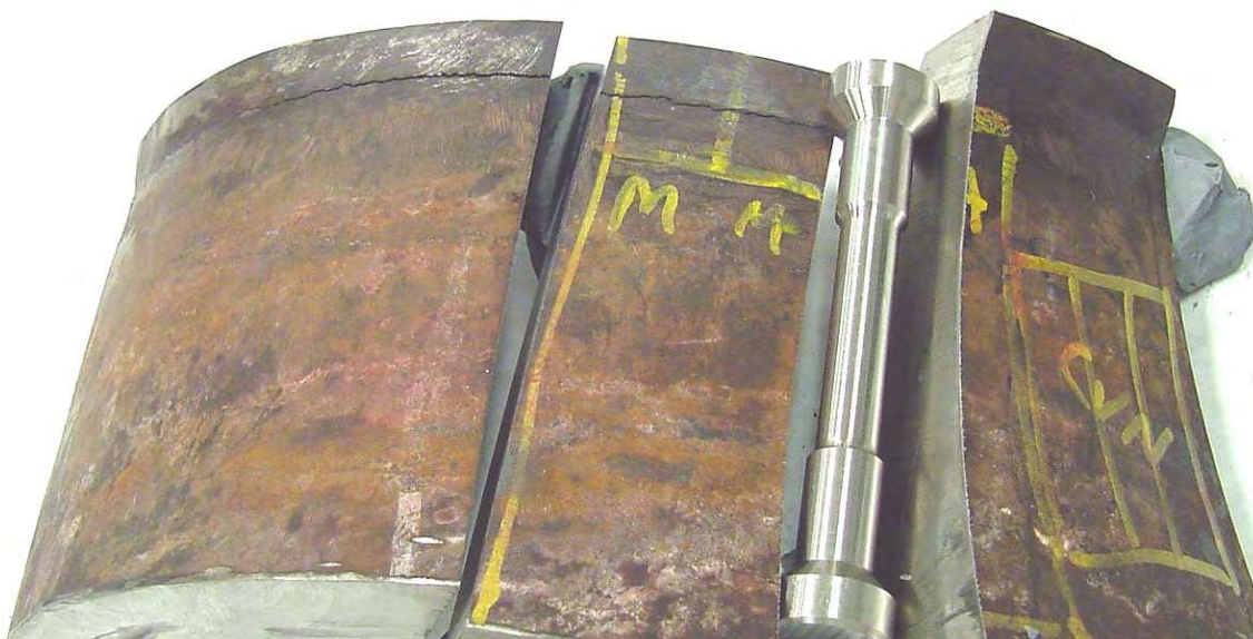
Figure 3-54-1—Samples removed from a cracked 12-in. NPS Type 321 SS elbow in a hot recycle H 2 line that operated at 985 °F (530 °C) in a hydrocracker.
