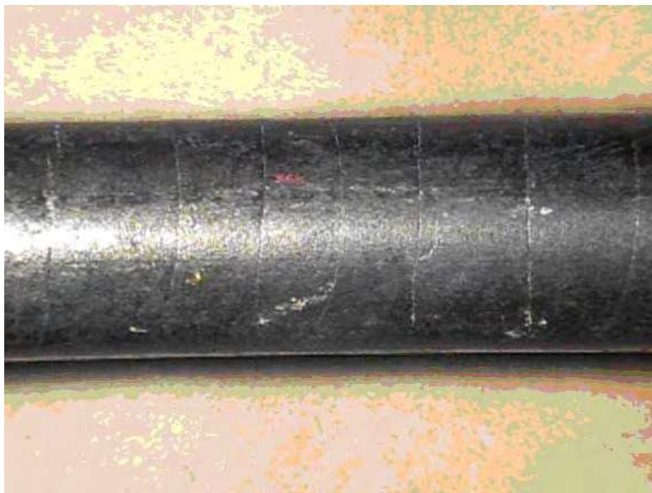
Figure 3-47-1—A nitrided 5Cr- \frac{1}{2} Mo thermowell tube from an ammonia synthesis plant with surface cracking.
