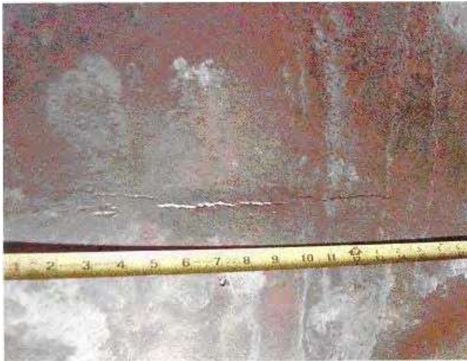
Figure 3-64-4—Thermal fatigue cracking associated with bulged skirt shown in Figure 3-64-3.
