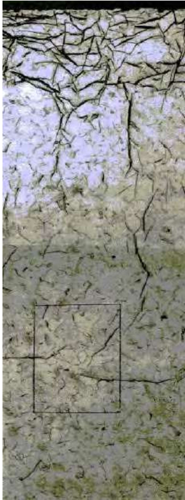
Figure 3-66-3—Another high-magnification photomicrograph of a cross section of the tube in Figure 3-66-1, showing more of the cross section through the tip of the crack. Titanium hydrides are more clearly discernable. Magnification 400X.
