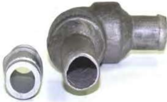
Figure 3-61-6—Sulfidation failure of a carbon steel sight glass nipple on the right after 2 years in a crude unit. Original thickness is shown on left for comparison. Material was supposed to be 9Cr-1Mo.
