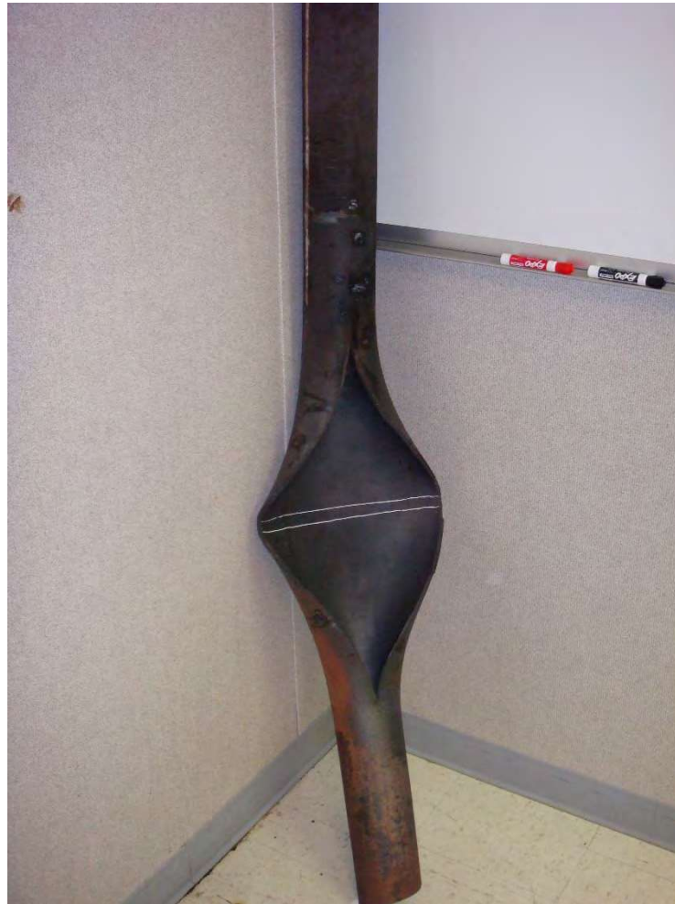
Figure 3-55-1—Short-term overheating failure of a vertical, 4.5-in. OD, schedule 160 2¼Cr-1Mo (SA335-P22) hydrocracker radiant tube that was 21 years old. Failure resulted from process-side starvation with the burners running.
