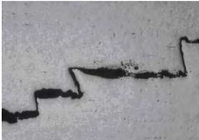
Figure 3-67-5—High-magnification photomicrograph showing stepwise cracking nature of HIC damage.
