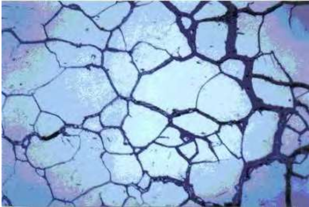
Figure 3-52-5—Higher-magnification view showing intergranular cracking. Magnification 200X.
