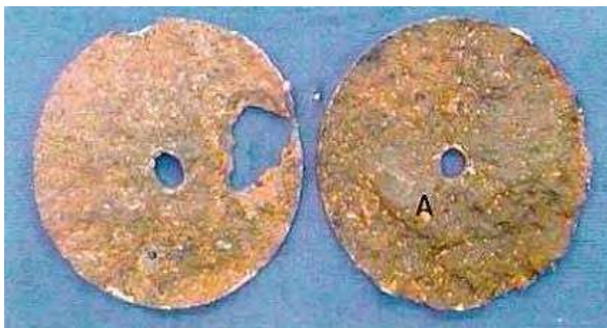
Figure 3-57-2—Coupons removed from the bottom of an unprotected steel condensate storage tank after 3 years of service. The external surface is shown.
